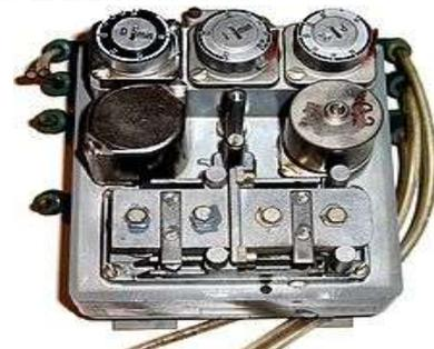
Figure 1 Three Term Pneumatic PID Controller
